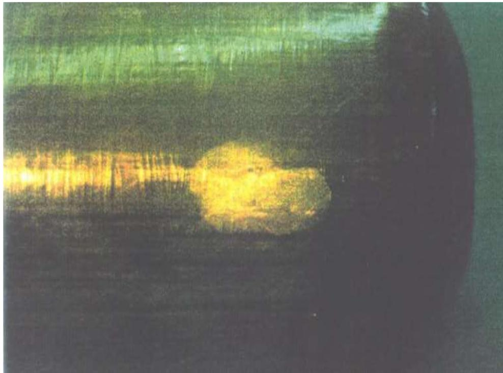
b) Level 3 impact damage — Depth of damage over 15 % of thickness (fully wrapped cylinder)
