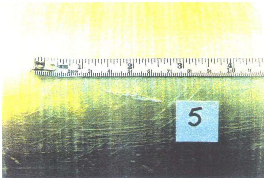
a) Level damage from cuts — Superficial cut
