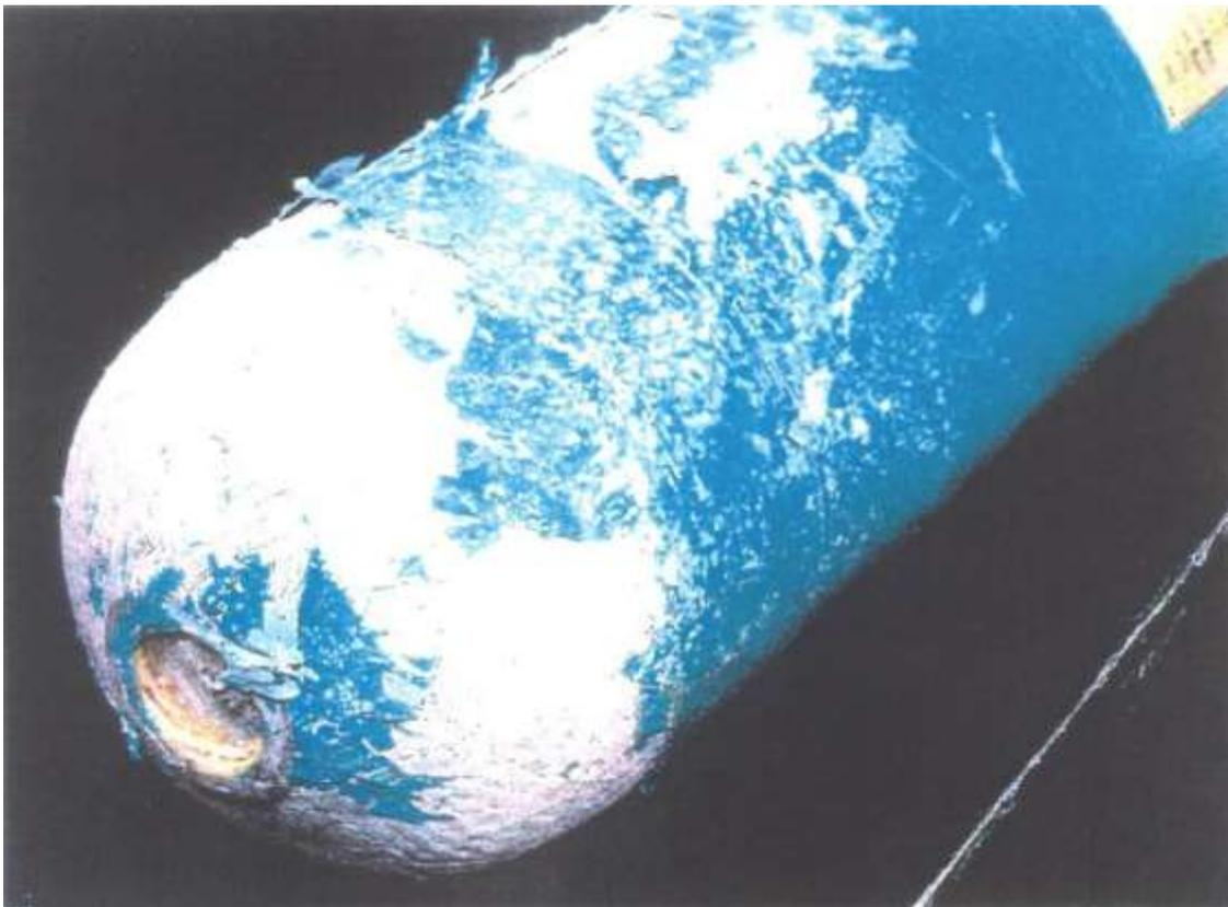
Figure 6 — Chemical attack (24 h in paint stripper)
