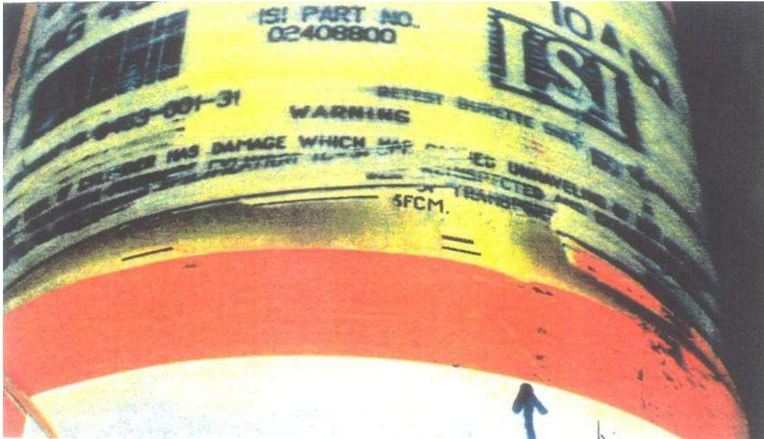
Figure 4 — Delamination
